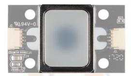
There is a marking next to the JST-SH connector that indicates polarity. The JST-SH connector breaks out the pins for serial UART and power. While the input voltage is between 3.3V and 6V, the UART's logic level is only 3.3V. It will need a logic level converter or voltage divider to safely communicate with a 5V device.
